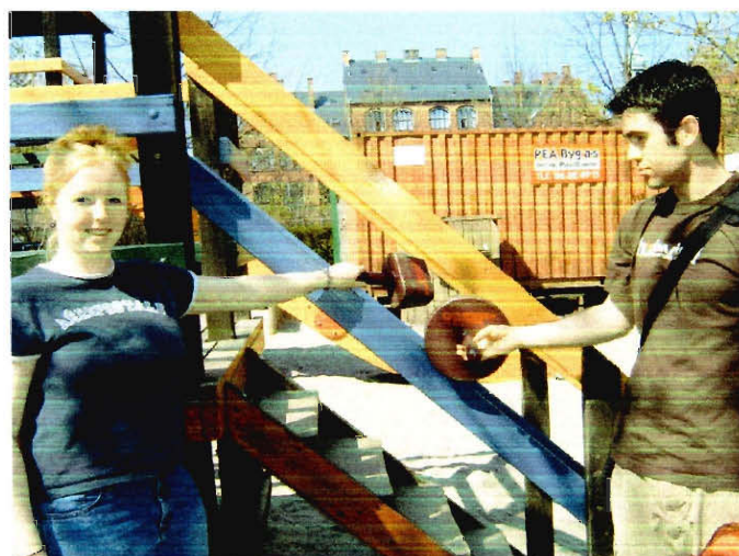
Fig. 4.14: Head Entrapment Test Failing on Handrails
