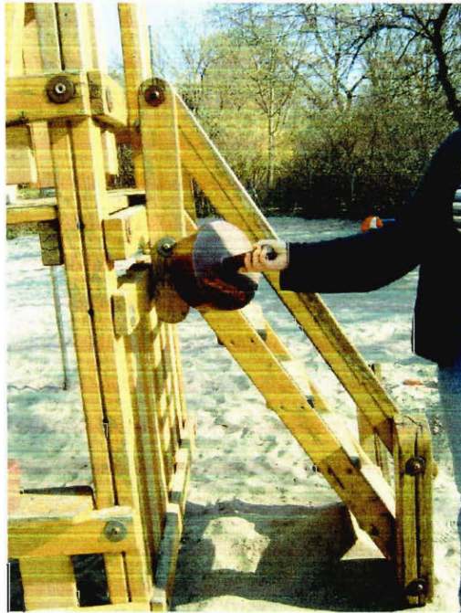
Fig. 4.23: Head Entrapment Test Failing on Handrail
