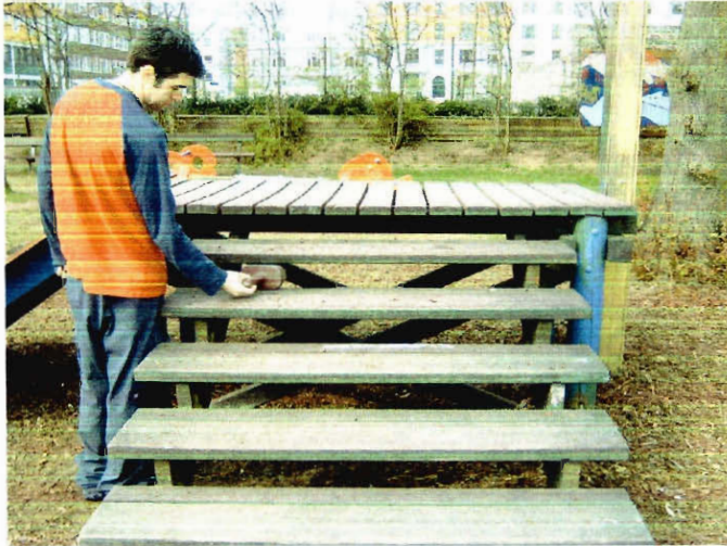
Fig. 4.27: Head Entrapment Test Failing on Stairs
