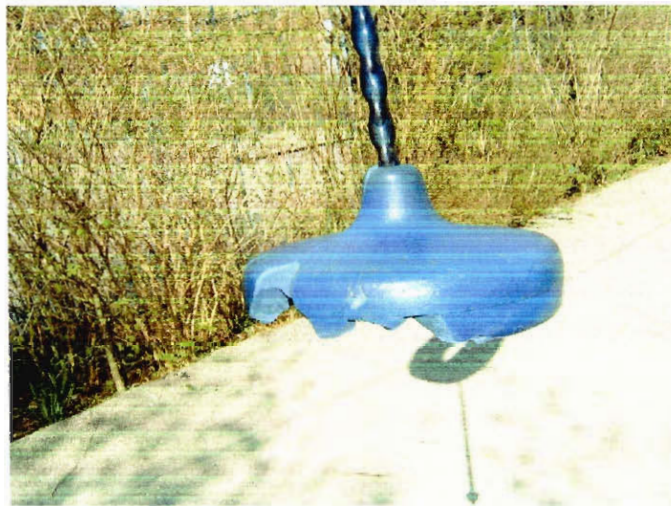
Fig. 4.20: Broken Zip Line Seat
