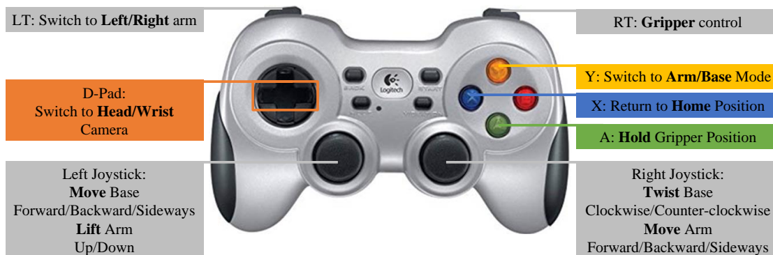
Figure 2.4: Gamepad controller configuration for teleoperation interface.
