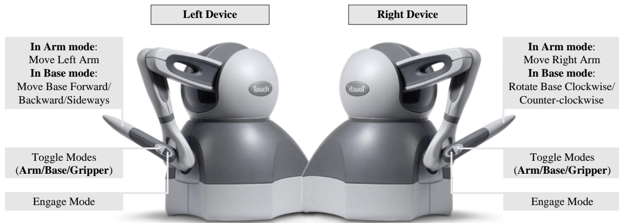
Figure 2.5: Stylus device (Geomagic Touch) configuration for teleoperation interface.
