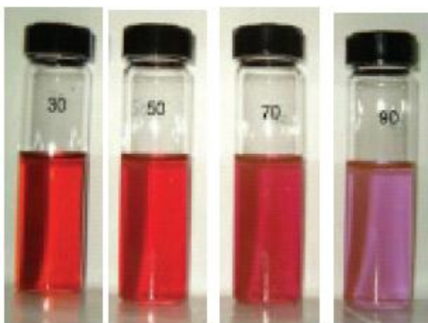
Figure 2.1: Color of nanoparticle solutions for different particle sizes[14]
