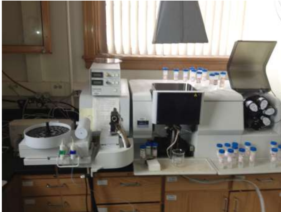
Figure 18: Atomic-absorption spectroscopy machine at WPI
