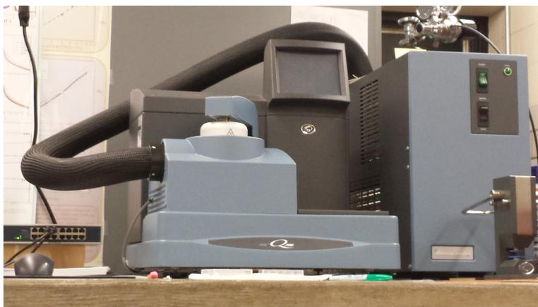
Figure 3.5: An image of the Q200 model Modulated Differential Scanning Calorimetry machine from TA Instruments.
