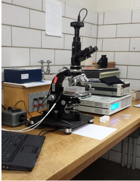
Figure 3.4: An image of a circa 1970 Labolux-pol Leitz Wetzlar microscope.
