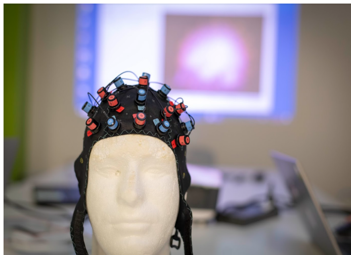
Figure 1. A picture of an fNIRS montage on an fNIRS cap. The montage is the series of red and blue optodes on top of the helmet/skullcap which is the fNIRS cap.
