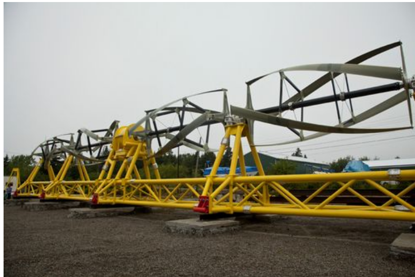
Figure 3.10 A Helical CFT being deployed in Cobscook Bay, Maine [15].
