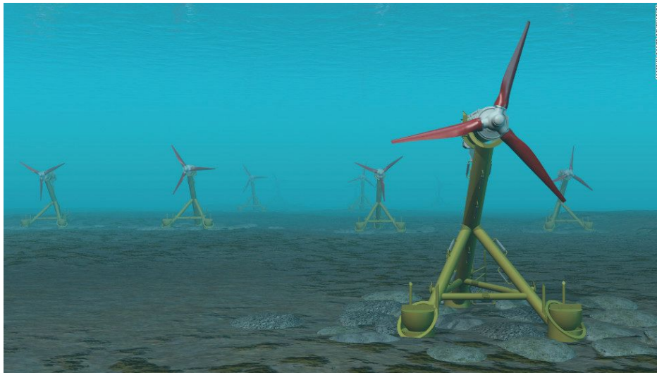
Figure 3.9 Axial turbine tidal generation [13].
