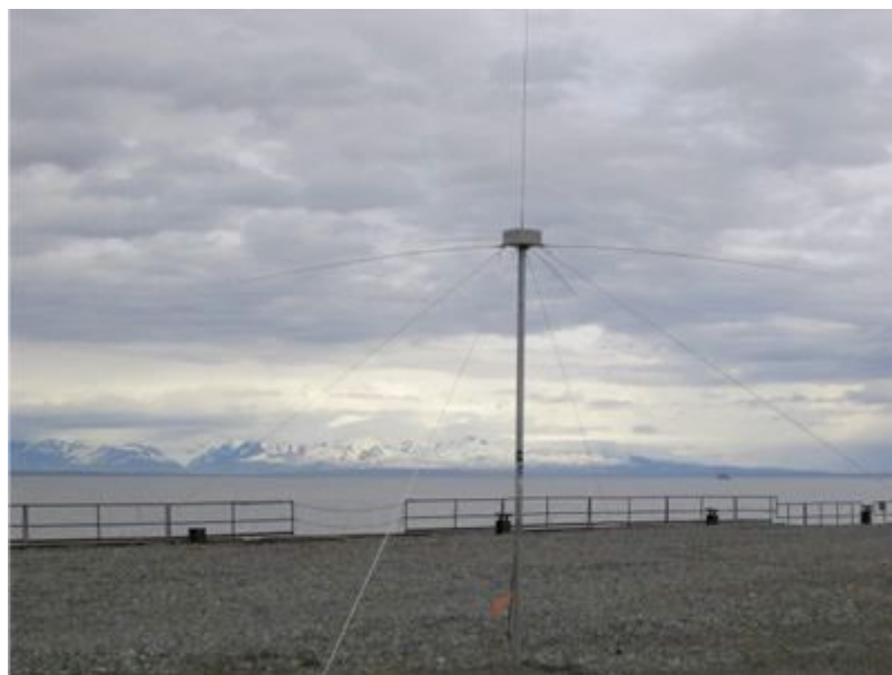
Figure 3.14 This is an antenna that used High Frequency radio signals to measure the speed and direction of the surface current using the Doppler effect [22].
