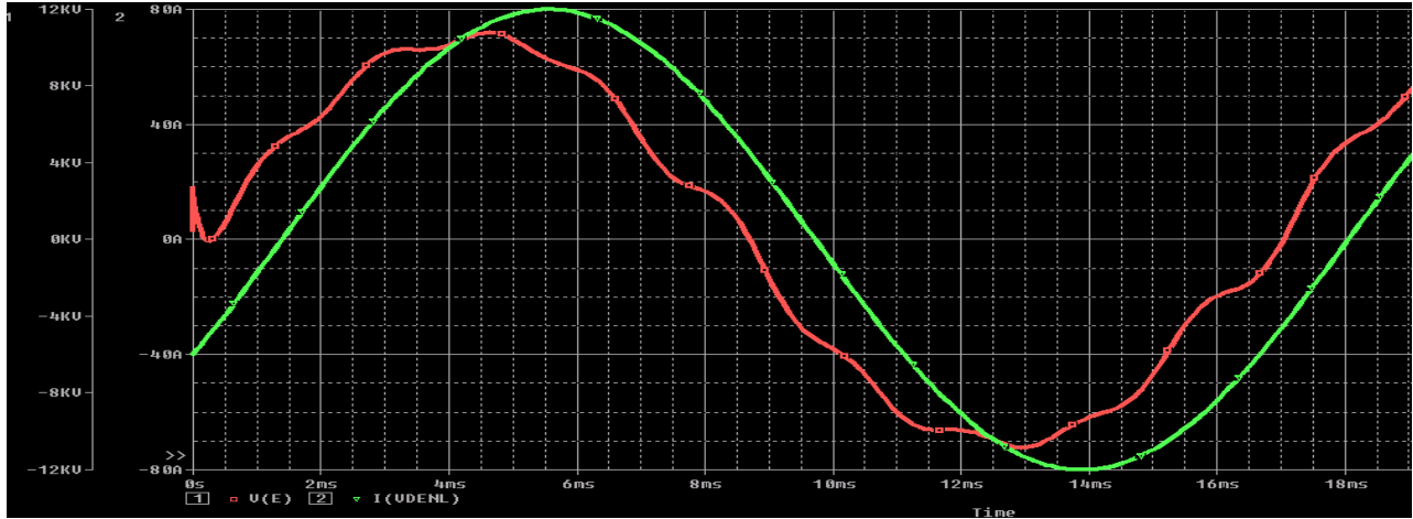
Figure 2-8 - Method II Current through the equivalent resistance at Node E. (green) Voltage at Node E (pink). Compensators at E and F and NLLs at H, I, and J.
