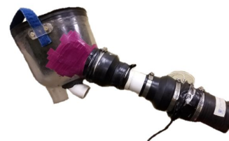
Fig. 1: Current Fleisch Pneumotachograph
