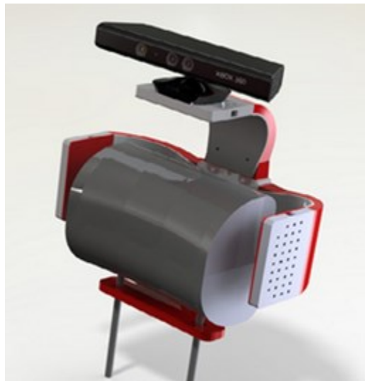
Figure 31: Headrest mount SolidWorks final design
