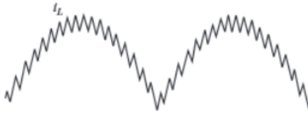
Figure 58: The current through the inductor [7]
