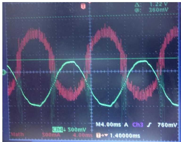
Figure 48: Voltage and Current Output from Transformer
