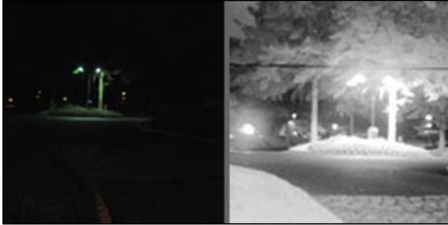
**Figure 15: SWIR camera being used for night vision (visible wavelength camera used on the left, SWIR camera used on the right) [17]**
