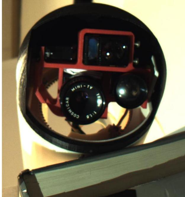
**Figure 62: Final Turret Design with Sensors**
