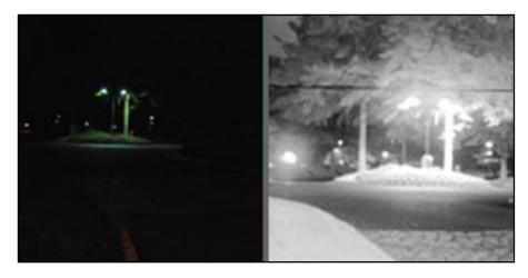
Figure 15: SWIR camera being used for night vision (visible wavelength camera used on the left, SWIR camera used on the right) [17]
