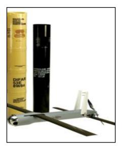
Figure 8: BAE Systems Coyote and its Sonobuoy Tube [9]
