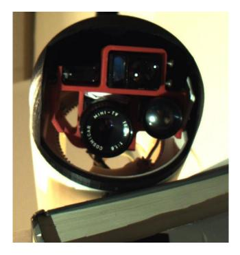
Figure 62: Final Turret Design with Sensors
