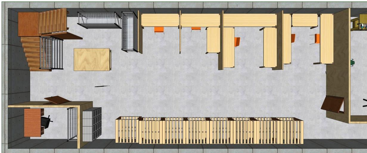
**Figure 2.8.** Storage and Extra Office Space design. This area must first accomplish the task of storing materials and member projects and personal items. Shelving is shown near the stairs for material and tool storage. Lockers are near the bottom left wall and pallets are along the bottom wall for rental storage. A small office was made for the facilities manager and all remaining space could be used for cubical space.
