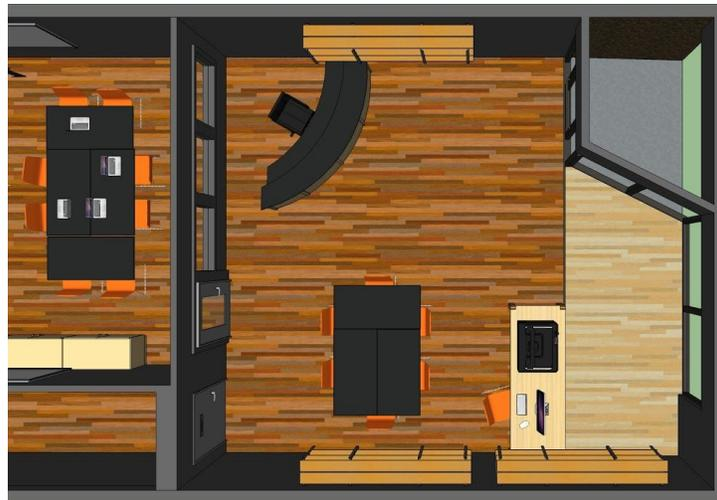
**Figure 2.2.** Reception area design. This area serves many purposes. The window area is a current structural feature of the carpet store; it should be used as a gallery space for the public to see. Tables and racks may be placed here as well for extra display space. A 3D printing station is also shown as an attraction. A reception desk and waiting/eating table should also be present.
