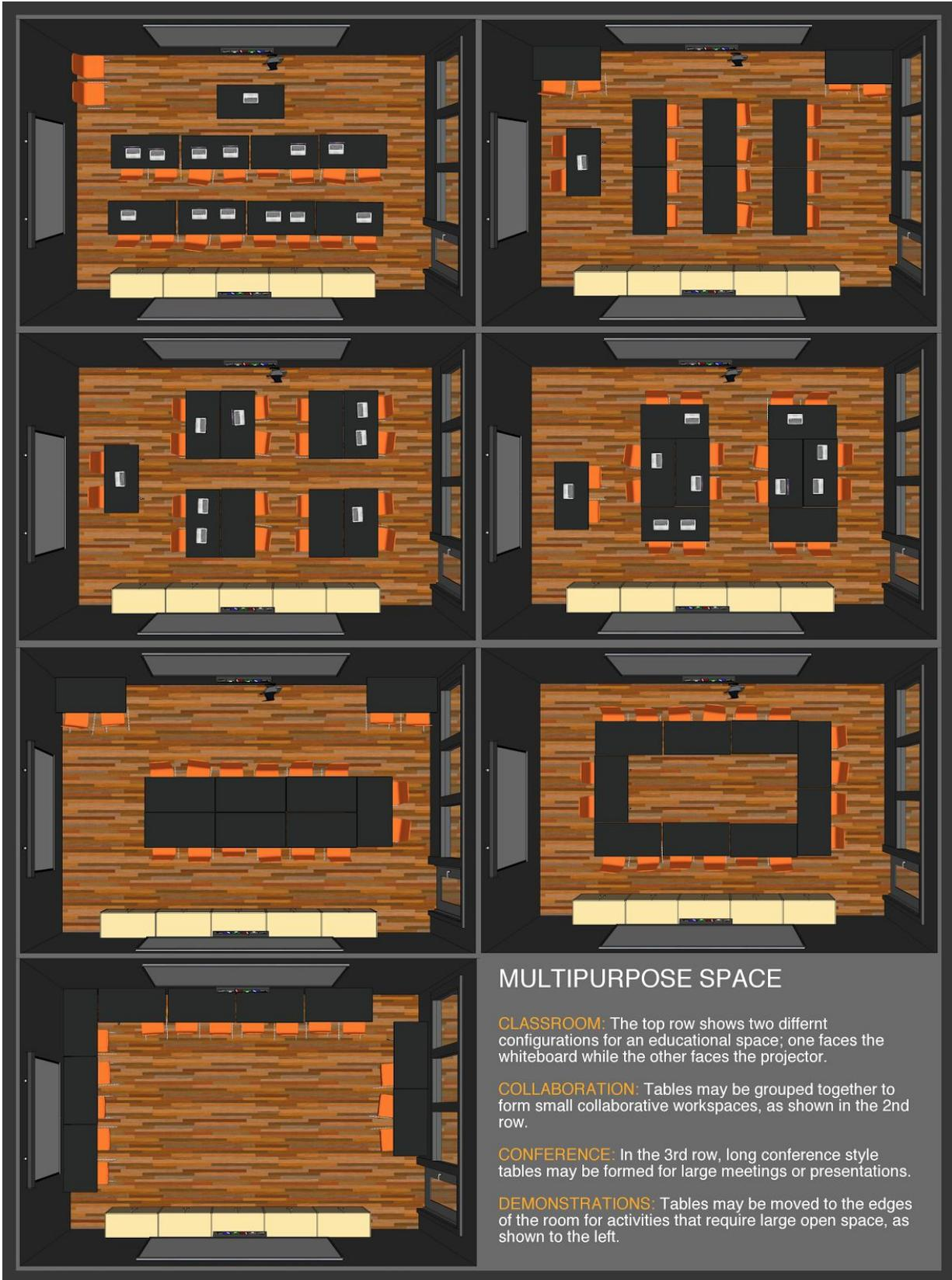
Figure 2.3. Possible multipurpose-space configurations. Mobile training tables are used to create any configuration desired.
