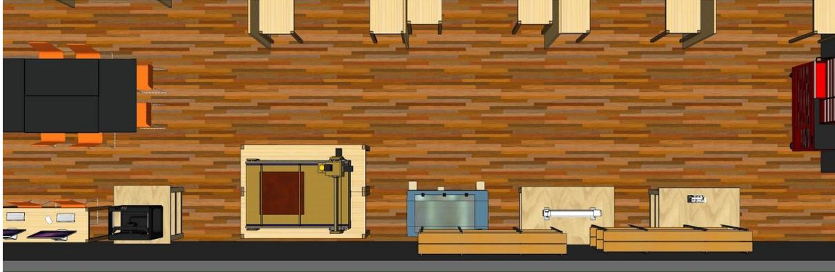
**Figure 2.5.** Prototyping and crafts space design. One or more sewing machines should be included. A vinyl cutter with plenty of spare fabric should be present in this space as well. For rapid prototyping, a laser cutter, CNC machine, and 3D printer are also shown.
