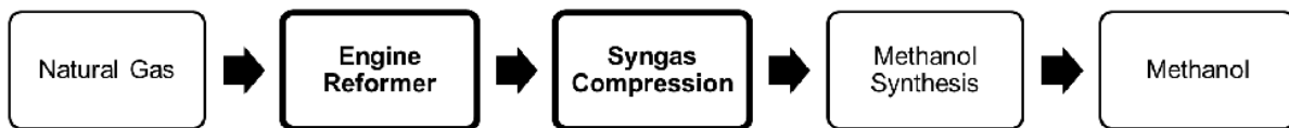
Figure 3. A block flow diagram from Dr. Browne's TEA on the gas-to-liquid (GTL) system utilizing an engine reformer (Browne, 2016).
