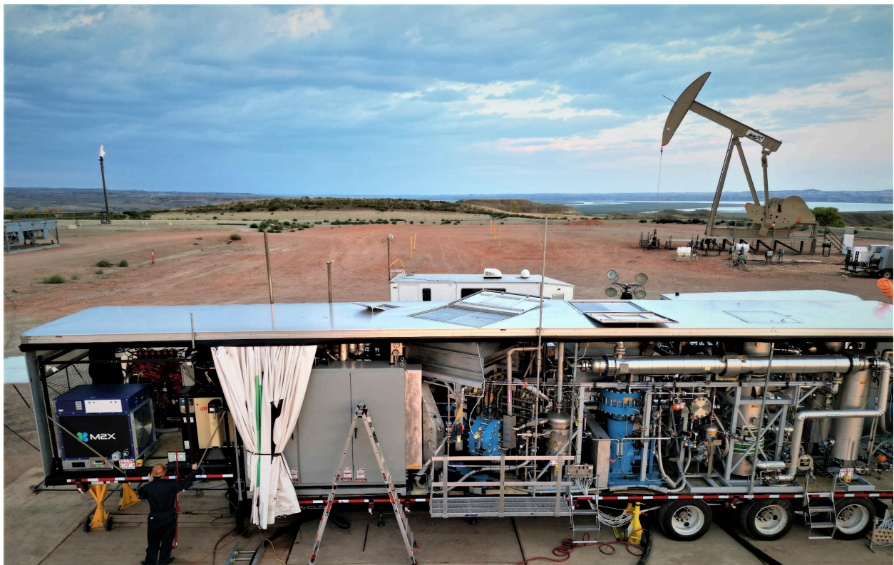
Figure 2. A full-scale skid unit of M2X's methane reformer technology at a test site in North Dakota (M2X Energy).
