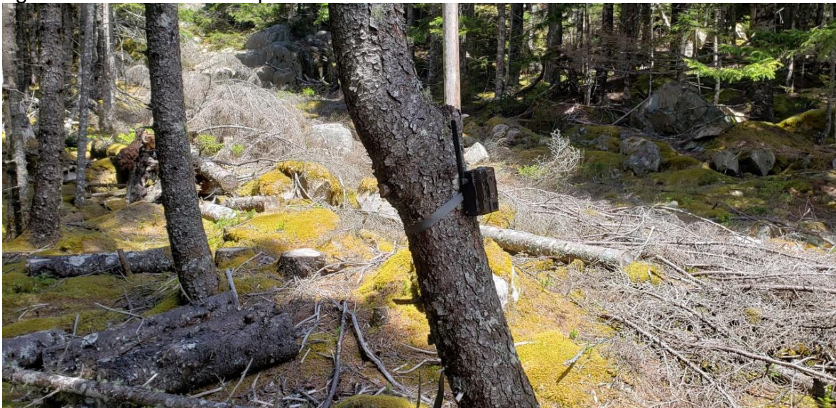
Figure 12: Link-Evo at First Location Secured to a Tree Using a Tree Strap
