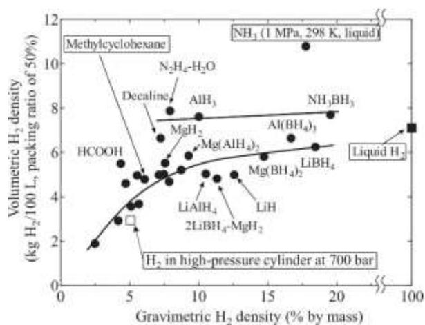
Figure 4. Gravimetric vs Volumetric Hydrogen densities (Kobayashi, H, 2019)
