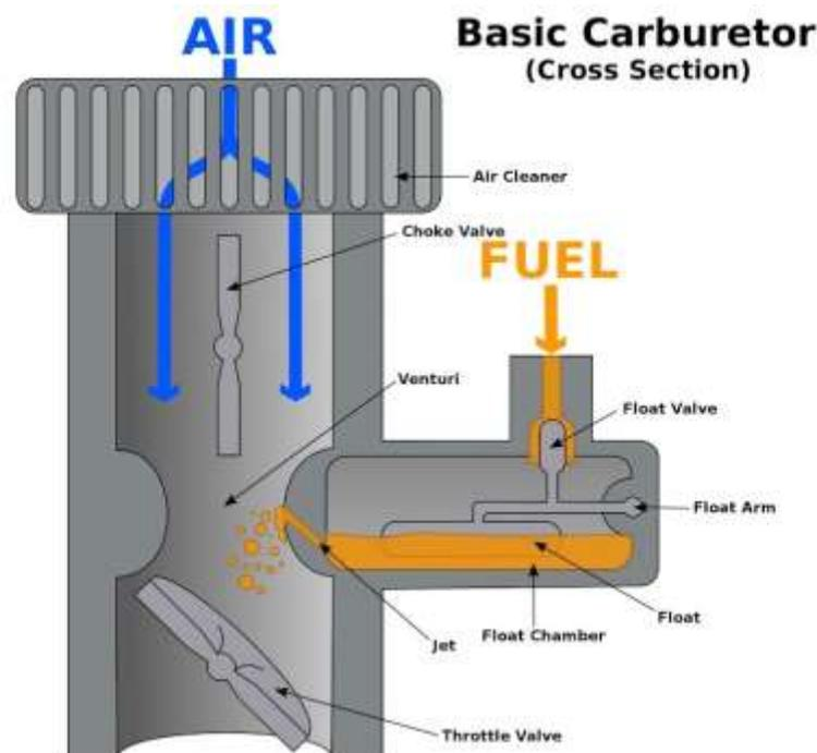
Figure 3. Carburetor Simplified
