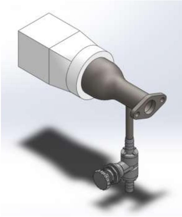
*Figure 7. NH<sub>3</sub> Carburetor Design*
