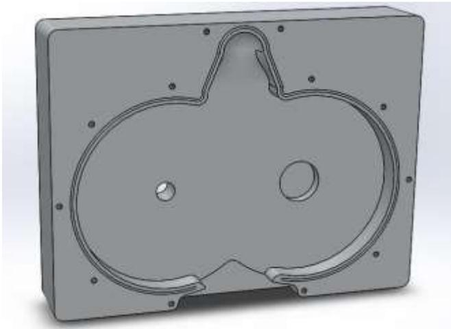
Figure 14. Dual Housing (Air Side)
