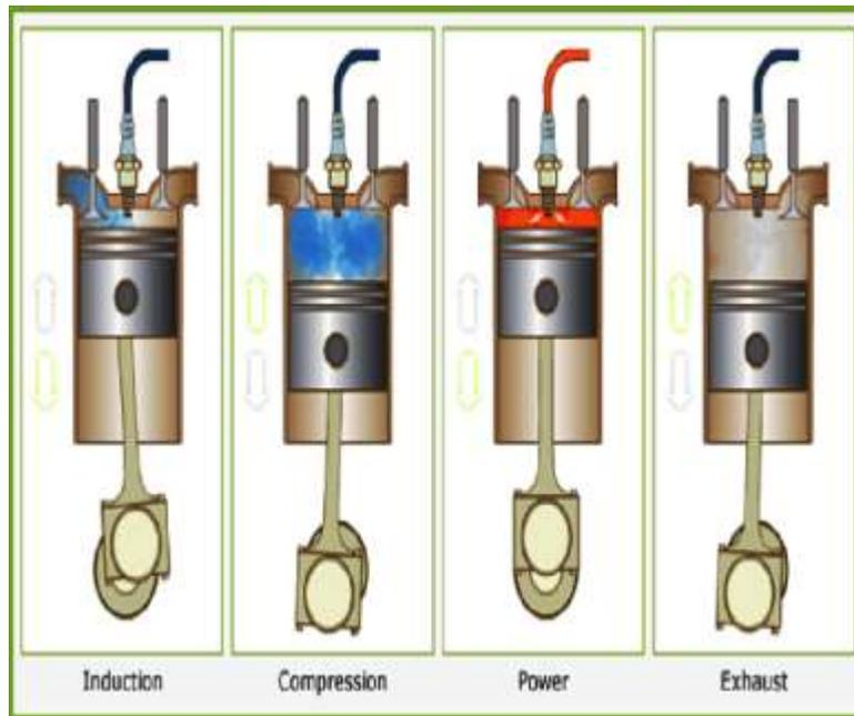
Figure 1. Four Stroke Diagram
