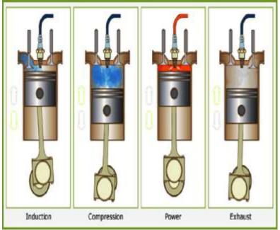
Figure 1. Four Stroke Diagram
