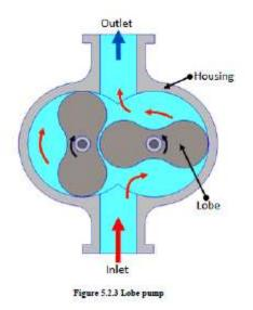
Figure 10. Positive Displacement Pump Diagram (Classification of Hydraulic Pumps. 2017. https://catengines.blogspot.com/2017/10/classification-of-hydraulic-pumps.html)
