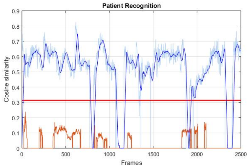
Figure 6.7: Similarity of the faces detected with respect to the reference face using a 10 element moving average filter in Scenario 1. Blue signifies the patient and orange marks the therapist. The red line is the threshold used to separate the patient from the therapist.
