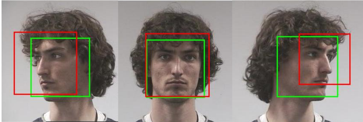
Figure 5.2: Example of face detection. In red the bounding box generated by HAAR Cascade algorithm and in green the bounding box generated by a deep learning model
