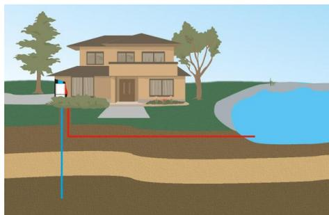
Figure 15: Geothermal Open Loop (GeoComfort, 2008)
