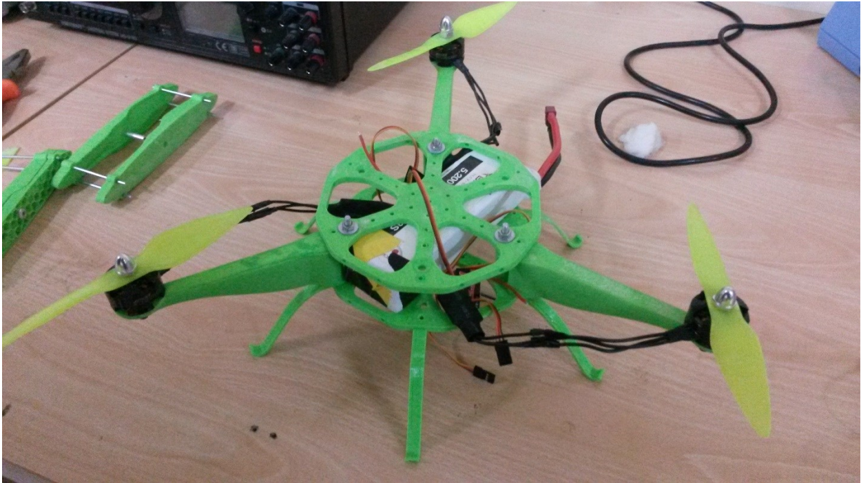
FIGURE 8.27: ASSEMBLED 3D PRINTED PARTS FOR DRONE GROUP
