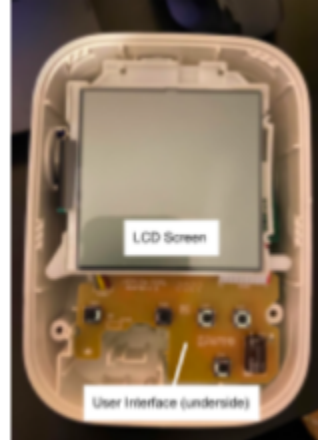
15B: OMRON Blood Pressure Monitor Interior User Interface Surface with Removal of Cover
