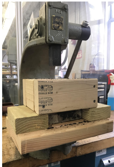
Figure 11: Arbor Press Compressing Blocks
