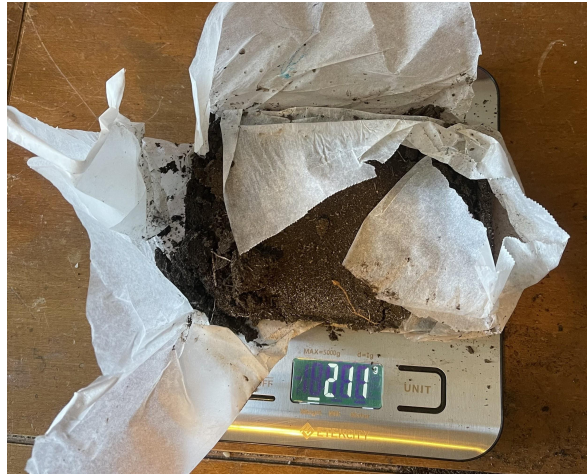
Figure 14: The Blocks During Density Test
