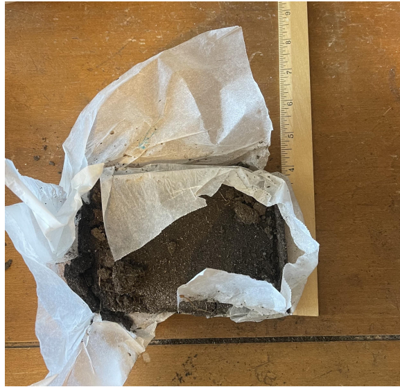
Figure 16: Block During Shrinkage Test
