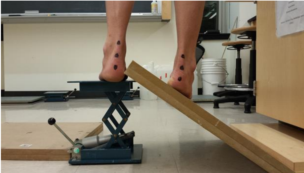
Figure 23: Group member on modified drop plate at 33 degree angle. Each subject stood on modified drop plate at 33 degree angle to measure ankle inversion.
