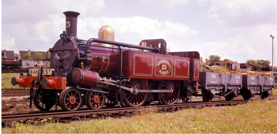
Metropolitan Railway A class 4-4-0T steam locomotive No. 23, 1866. Taken from the London Transport Museum's Online Collection (Reference: 1998/37950)
