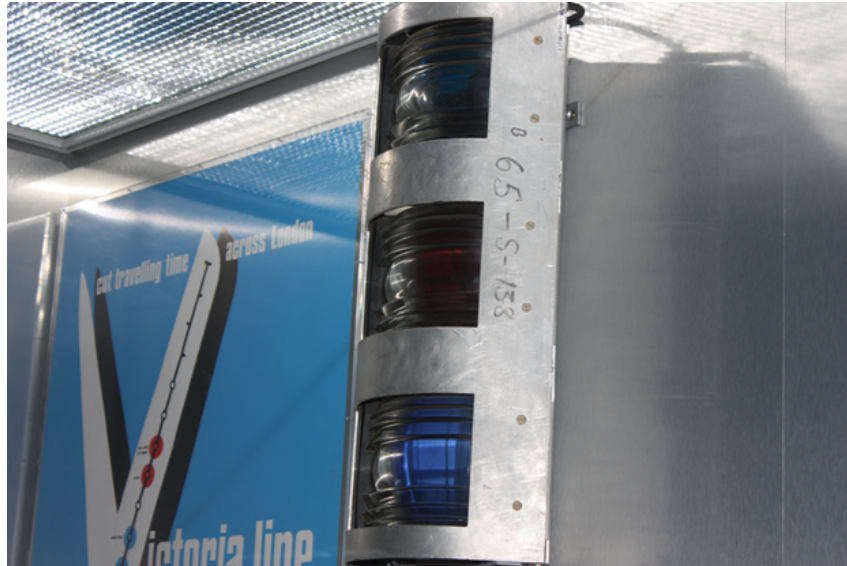
A multi-aspect signal from the Victoria line on display at the London Transport Museum (LTM).
