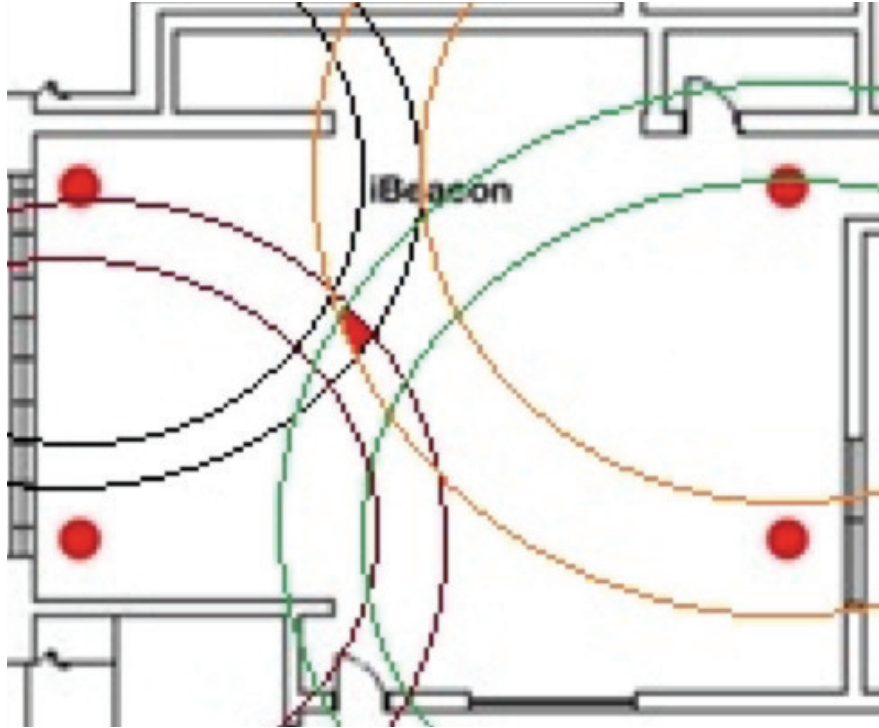
Figure 4.4: Algorithm of In-Room Localization.
