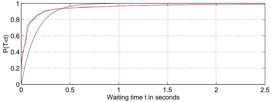
Figure 22: Erlangian Fit of Interarrival Times
