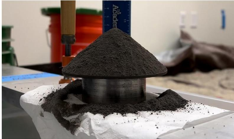
Fig. 4.33 JSC-1 Regolith Simulant Angle of Repose Testing.
