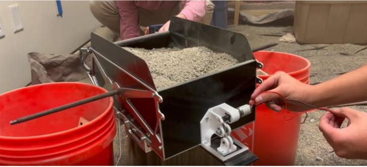
Fig. 5.11 Deposit Yoke Mechanism Activated.
