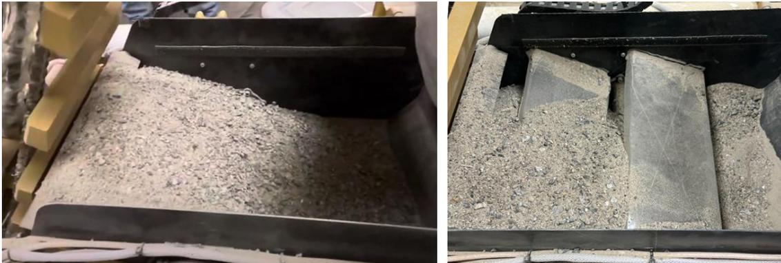
Fig. 6.3 Left: Initial material distribution. Right: Material distribution with louvers.
