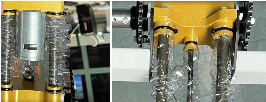
Fig. 4.27 Bellows attachments on Static and Upper blocks.
