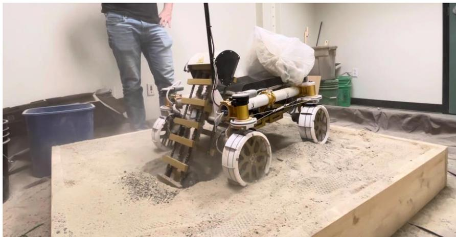
Fig. 5.17 Berm Construction Test, digging cycle.
