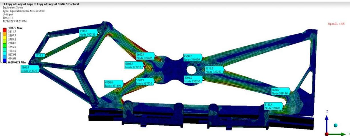
Fig. 4.39 Aluminum Structural Analysis Results.
