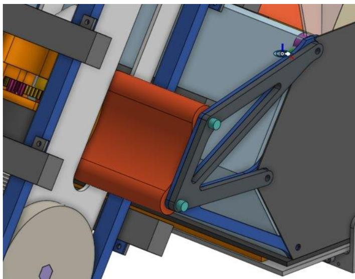
Fig. 4.40 Conveyor Attachment Point.
