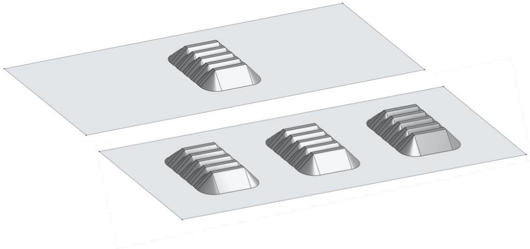
Fig. 4.17 Regolith pile(s) in the berm zone for minimum and reach goals.
