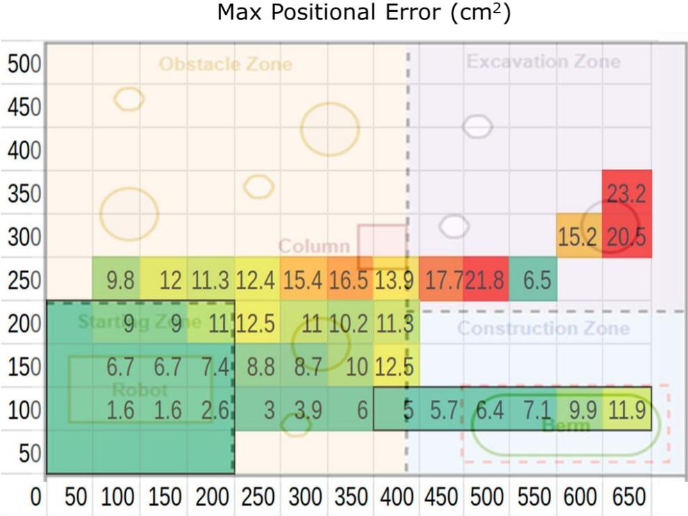
Fig. 5.14 Localization ArUco Testing.
