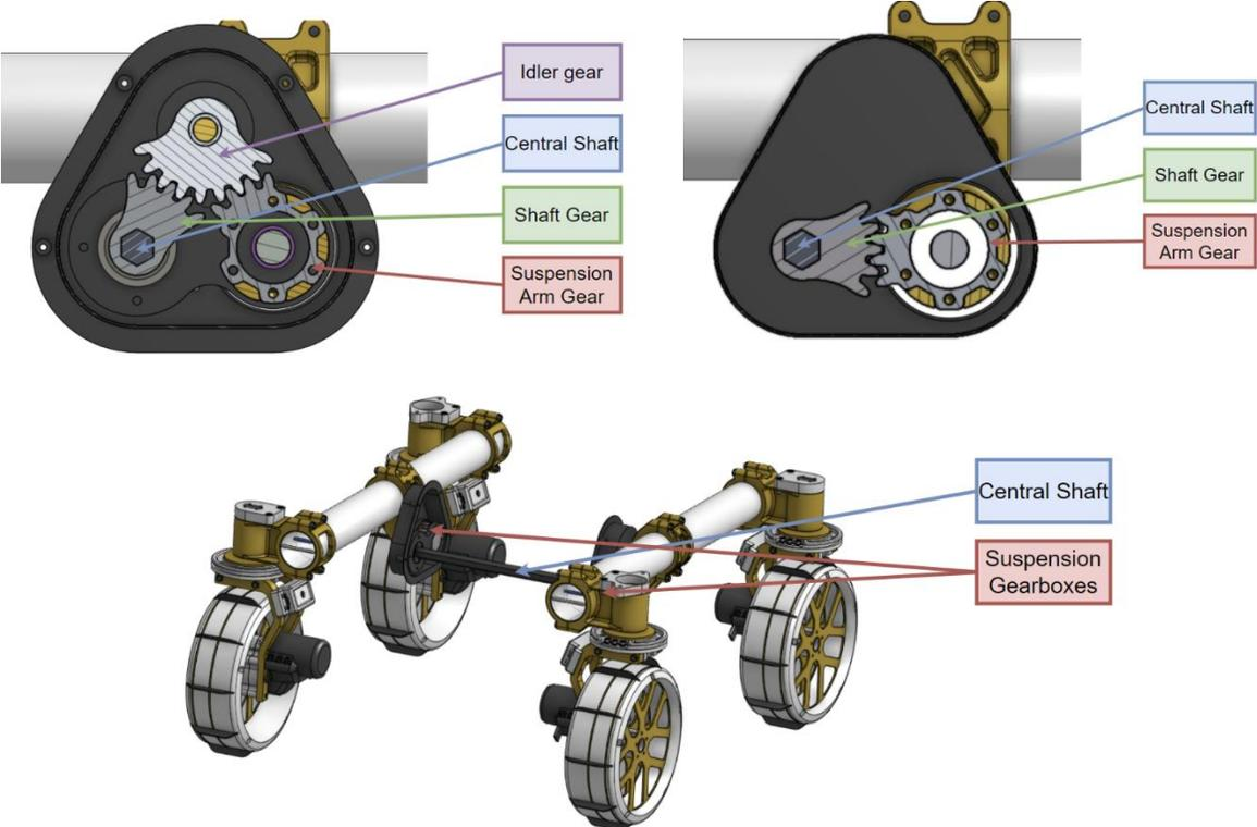
Fig. 4.13 Geared Rocker Suspension.
