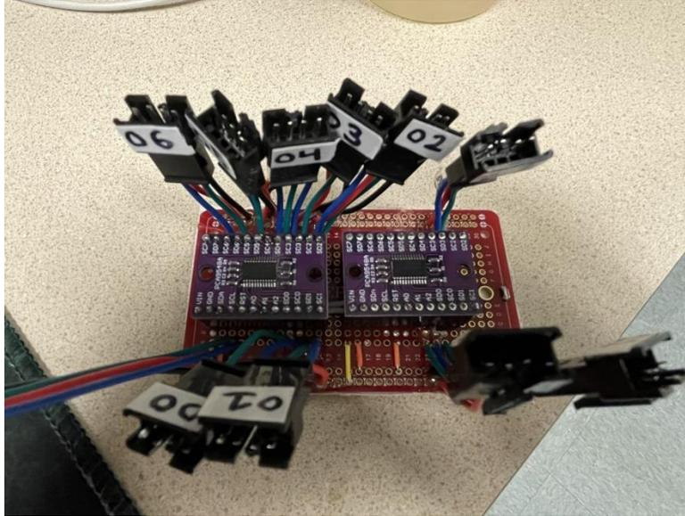
Fig. 4.56 Multiplexer Array.
