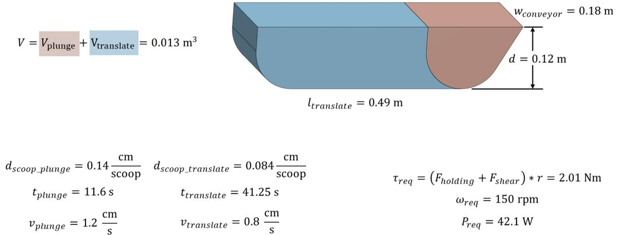
Fig. 4.24 The plunging/translation volumes allow us to exceed our minimum regolith goal in one digging cycle.
