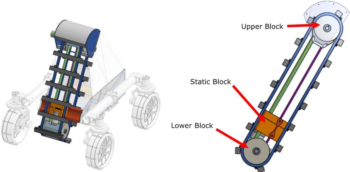
Fig. 4.21 Regolith Intake System.
