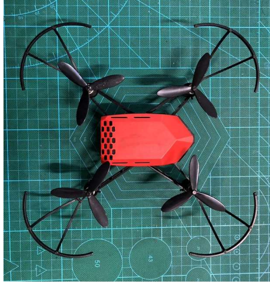
Figure 17: R130 viewed from the top. Battery pack and propeller guards attached. Specification sheet in Appendix J .
