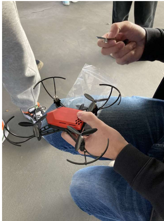
Figure 19: Picture of team member replacing propeller in about one minute.
