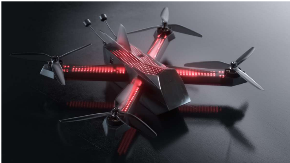
Figure 5: The DRL Racer4 drone. Clean look with bright LED lighting. Classified as a rotary-wing MAV quadcopter; four propellers give balance between practicality and efficiency (Source: Bleier, 2019).
