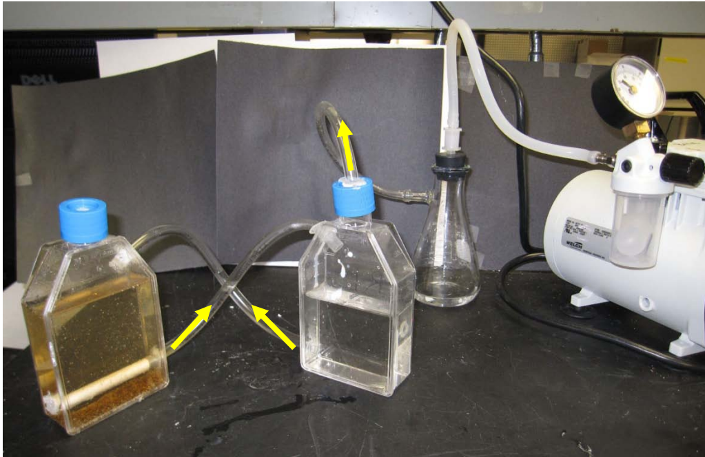
Figure 21: Recirculating media system.
