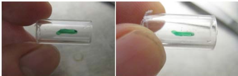
Figure 28: PETG control (unseeded) mandrel with indicating line for determining cellular adhesion (left image). The image on the right is the same mandrel, rotated 180 degrees.
