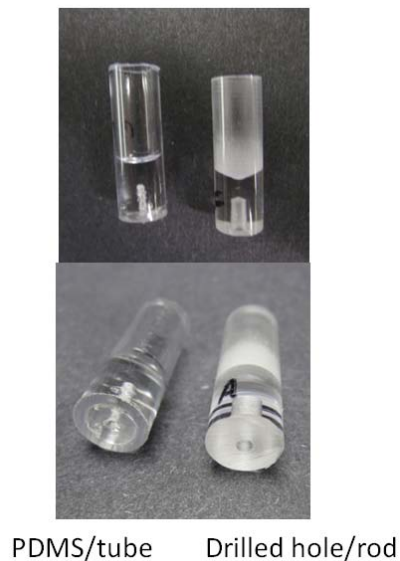
Figure 42. The previous mandrel fabrication involved PDMS casting into a tube, while the new method involved drilling a hole into a rod creating a much more stable connection to the motor
