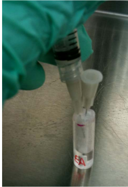
Figure 60: Method for insertion of cell suspension into tube.
