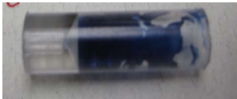
Figure 54: Results of Experiment 5 showing Trypan blue staining of polycarbonate after 15 minutes spinning with 25 million cells.
