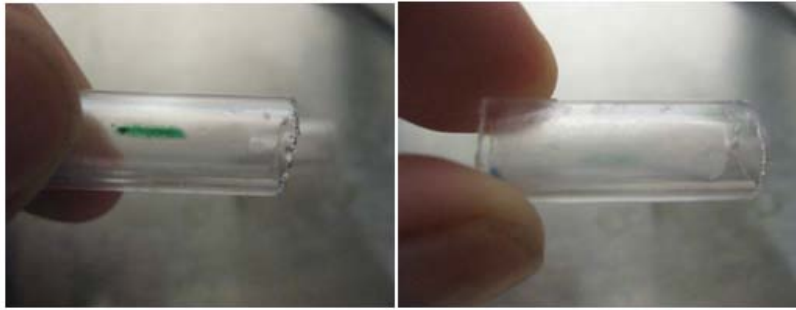
Figure 27: PETG mandrel with indicating line for determining cellular adhesion (left image). The image on the right is the same mandrel, rotated 180 degrees.
