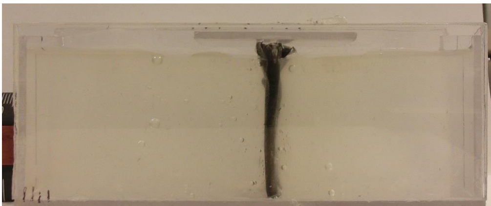
Figure 30: Collapsed PTFE Sheath in Gel
