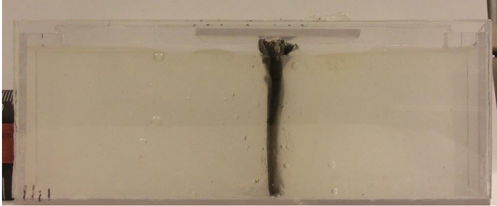
Figure 26: Collapsed PTFE Sheath in Gel
