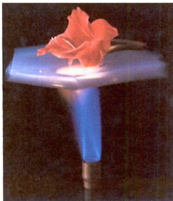
Figure 5.1- Flower Protected from Flame by Aerogel
