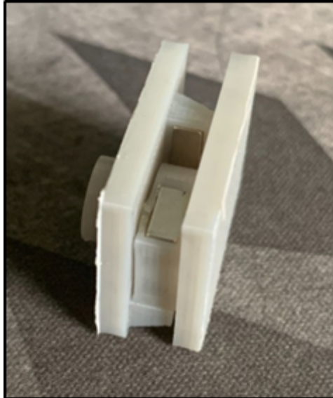
Figure 77. 3D Printed Hot End Swivel V1 Magnet Slots
