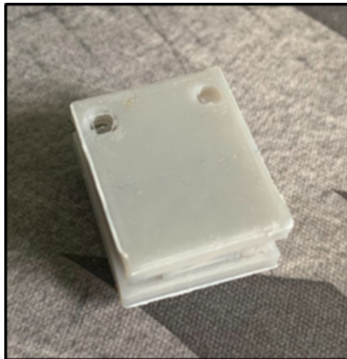
Figure 76. 3D Printed Hot End Swivel V1
