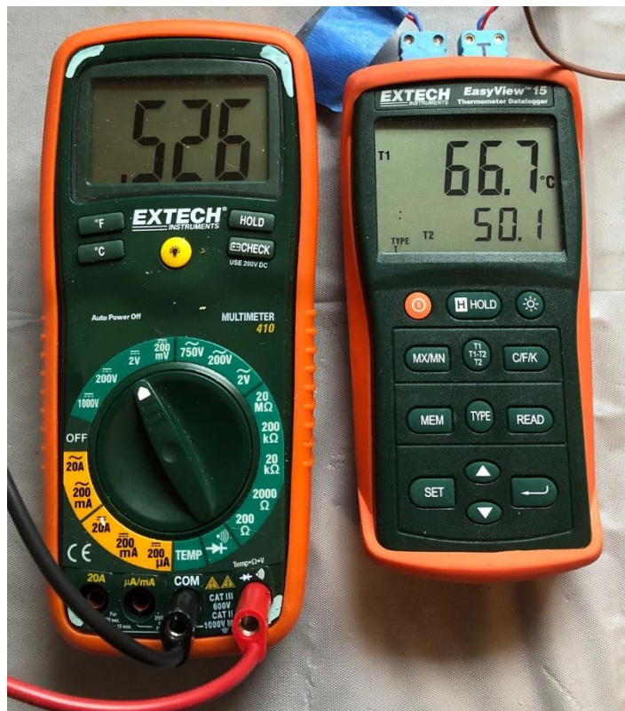
Figure 16: EXTECH 410 Multimeter (left) and EXTECH Thermocouple Datalogger (right)
