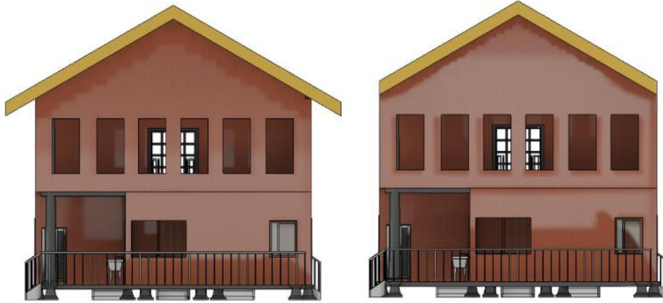
Figure 26: Example of roof with no overhang and one meter overhang on the design.
