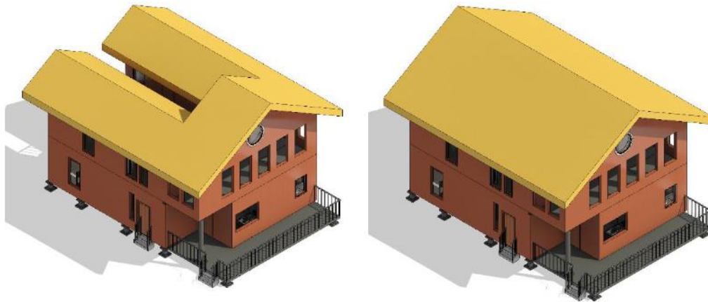
Figure 13: Comparison of one extensive truss system and three smaller sectioned truss systems.
