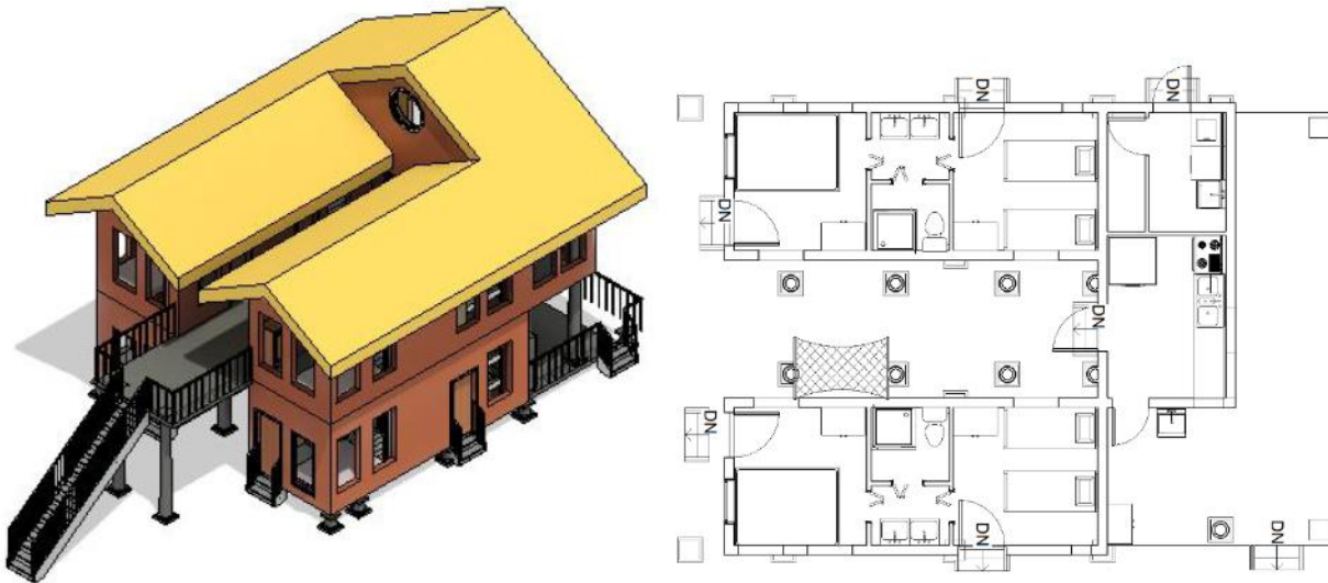
Figure 6: Final design draft of the dormitory space, inclusive of a kitchen, balcony, and deck.
