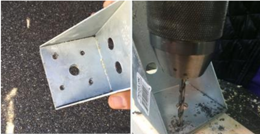
Figure 55 Drilling Holes in Corner Bracket
