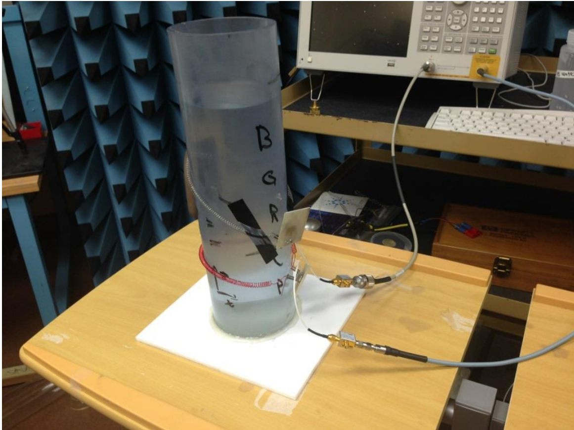
Figure 33: Coil Antenna Setup
