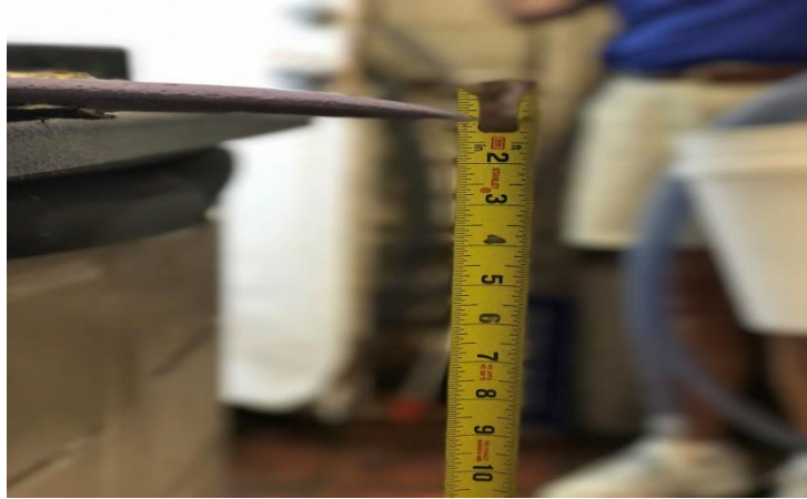
Figure 25: Flipper currently being used at the aquarium deflecting 1 inch.
