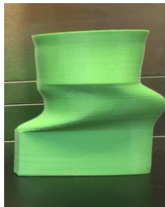
Figure 18: The 3D printed piece used to create the mold for the final design.
