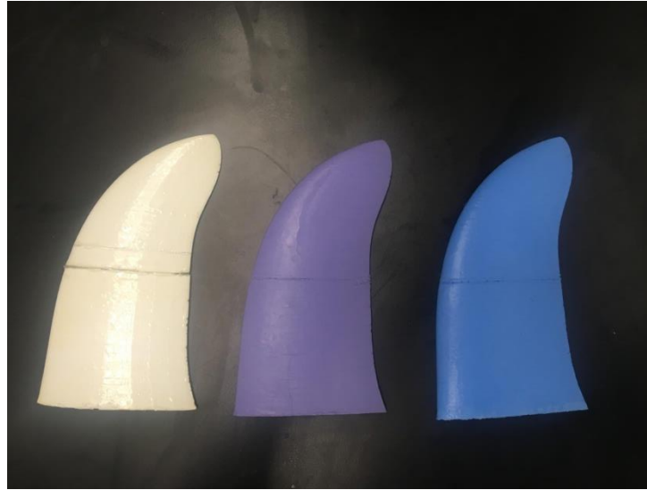
Figure 17: 3D printed flipper blade; Smooth-Sil 945 flipper blade; Smooth-Sil 950 flipper blade.
