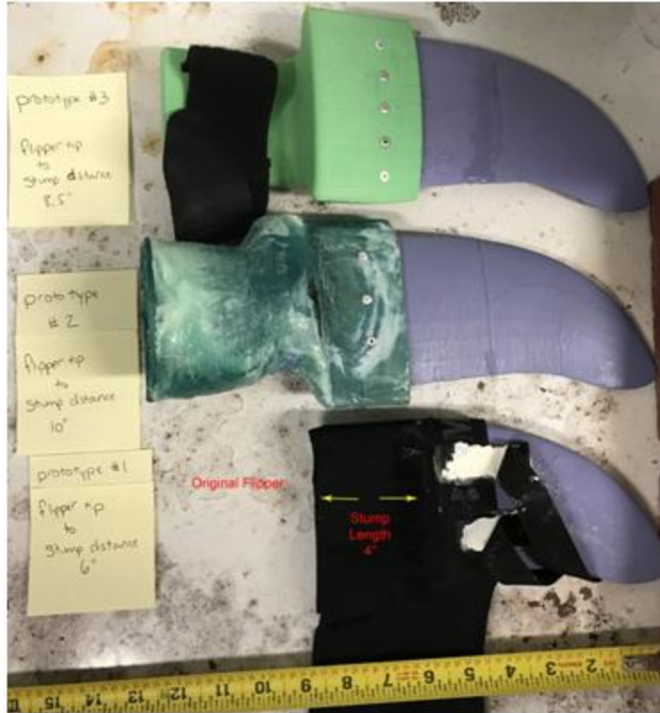
Figure 37: (T-B) Loop and Plate Design, Shuttle Lock Design, and Previous Design Prostheses Lengths.
