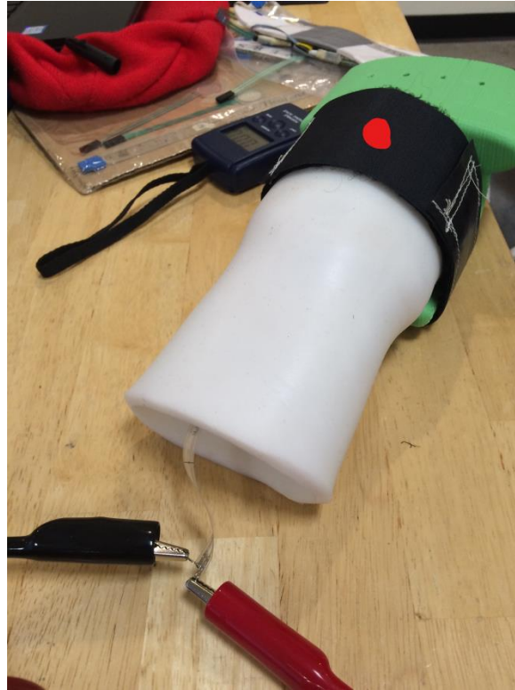
Figure 30: Pressure testing of Loop and Plate Design.
