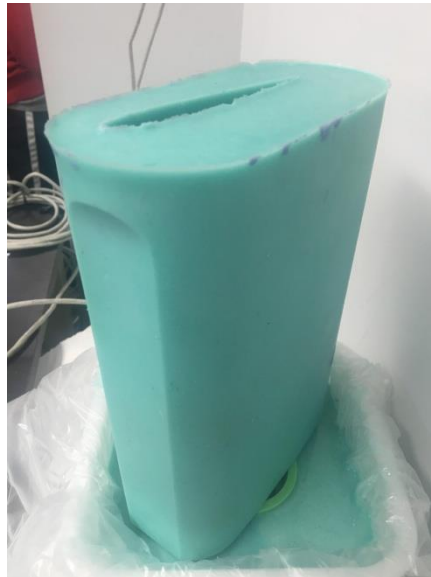
Figure 16: Negative mold of the 3D printed flipper blade.
