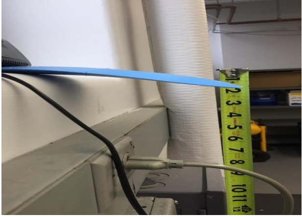
Figure 23: Flipper made of Smooth-Sil 950 deflecting 1.5 inches.
