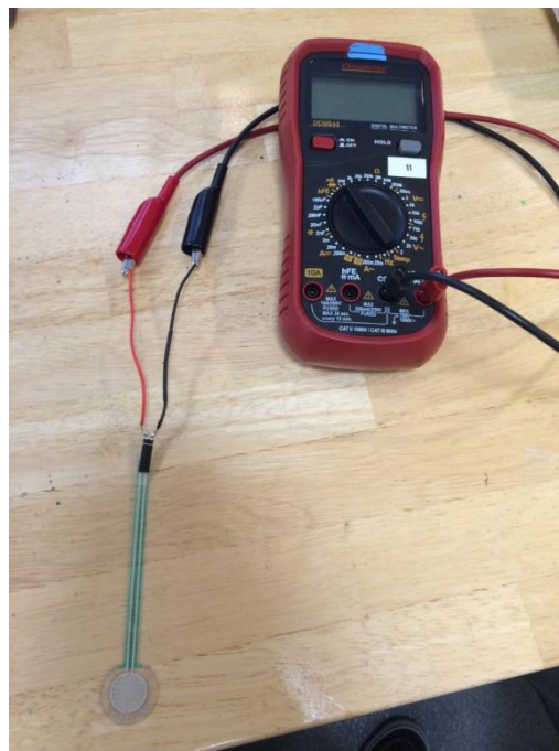
Figure 27: Setup for pressure testing.
