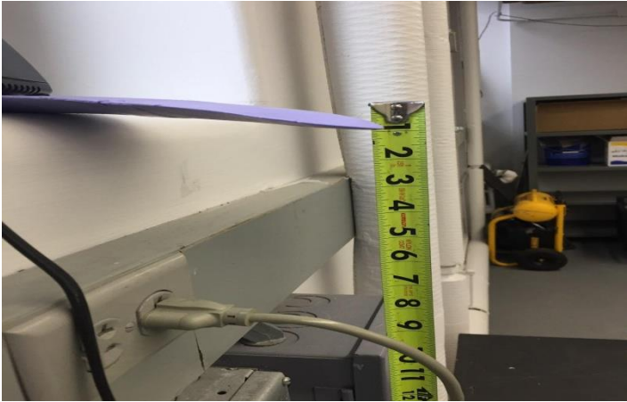
Figure 24: Flipper made of Smooth-Sil 945 deflecting 1 inch.
