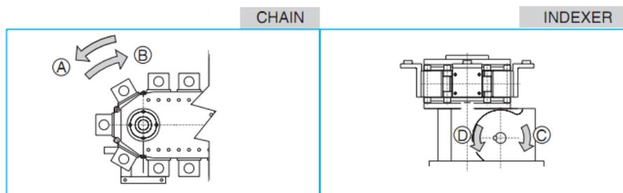
Figure 1: Indexing motion in a precision link conveyor system.
