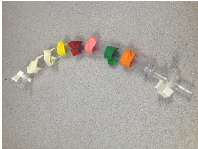
Figure 28 Same-Time filling of tiered Balloon catheter
