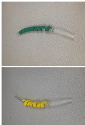
Figure 31 Tightly wrapped cylindrical prototype (top) and loosely wrapped cylindrical prototype (bottom).
