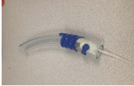
Figure 30 Cylindrical balloon wrapped around wide catheter tube
