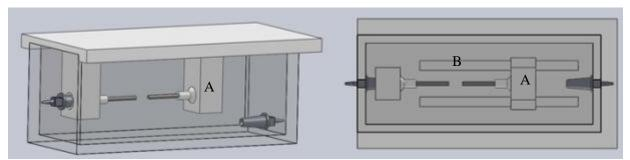
Figure 15: The first iteration of the sliding track design. A sliding T-shaped arm (A) moved along tracks (B) in order to adjust the positioning of one of the syringe needles.
