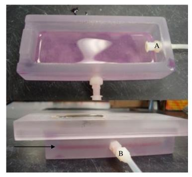
Figure 39: The cell media evaporated which did not allow the cell media to contact the inlet Luer (A). The cell media just barely reached the outlet Luer (B). The level of media is indicated by an arrow in the side-view.
