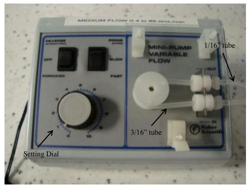
Figure 23: Fisher Scientific peristaltic pump with flow rates ranging between 0.4-85.0mL/min.
