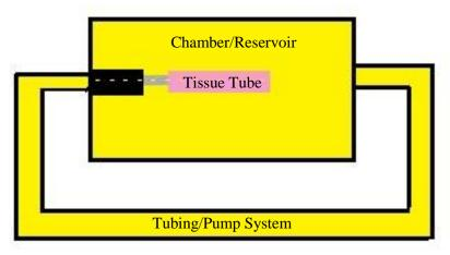
Figure 8: The "one media chamber" design consists of a chamber that acts as the media reservoir as well as the area where the tissue sample is submerged. The same media is circulated through the lumen as well as around the outside of the tissue tube, indicated by the single color of the media.
