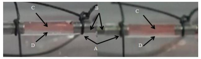
Figure 36: The silicone tubing is sutured (A) to the syringe needles (B). The red food coloring makes a visible, distinct layer (C) above the clear water (D).
