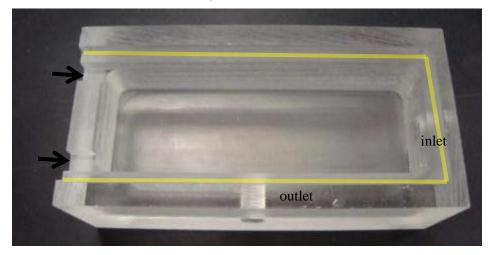
Figure 21: Acrylic prototype chamber with edges for lid (highlighted in yellow) and slots for ridges on lid (labeled with arrows).
