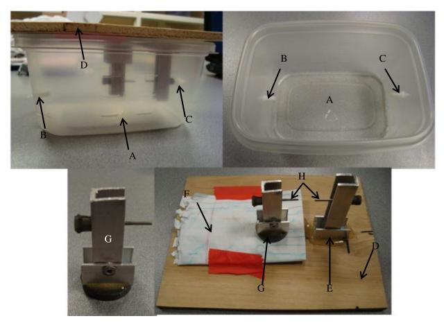
Figure 18: The initial prototype consisted of a Tupperware® container (A) with outlet (B) and inlet (C) Luers, a wooden board (D) acting as the lid with a stationary aluminum arm (E) and steel track (hidden by the paper labeled by F), and a magnetic aluminum movable arm (G). Both arms have aligned syringe needles (H). The paper was used to even out the height of the movable arm.
