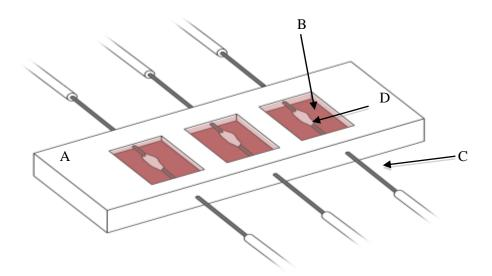
Figure 6: Top View Bioreactor Schematic of the design by Lovett *et al.* (2007). Labeled are the PDMS block (A), the media-filled wells (B), steel needles for perfusion (C), and the tissue tube mounted on the needles (D).
