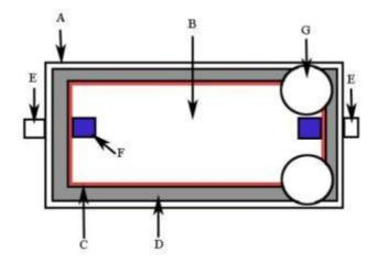
Figure 4: Growth cassette developed by Webb *et al.* (2007) which includes the cassette body (A), plexiglass faceplate (B), rubber gasket (C), aluminum frame (D), flow inlet/outlets via Luer connectors (E), Luer connector for scaffold attachment (F), and an air filter for gas exchange attached to a Luer connector (G).
