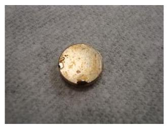
Figure 58: Magnet after it was removed from the movable arm. The nickel appears to be chipped causing it to rust.
