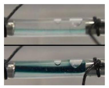
Figure 38: Laminar flow shown by upstream injection of food coloring. This image shows a thin stream (A) as well as a thick steam (B) showing no signs of turbulent flow.
