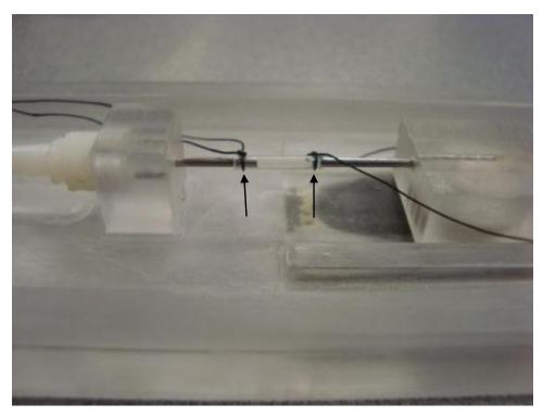
Figure 30: Silicone tube mounted onto the syringe tips using medical sutures (arrows).
