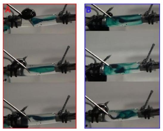
Figure 37: Flow patterns that resembled laminar flow (A) and turbulent flow (B).
