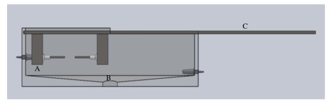
Figure 14: Lunchbox Design with sliding Luer connection (A), sloped bottom for draining media (B), and sliding lid with long handle (C).
