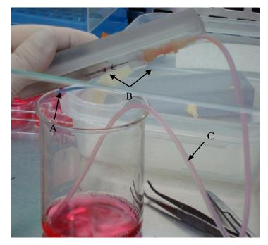
Figure 35: Media flows all the way through the tissue tube and comes out the end of the movable arm (A). No leaking is observed at the tissue-syringe interface or the Luer-tubing interface (B). Media flows from a beaker through the tubing and into the arms of the lid, priming the tubes in the process (C).
