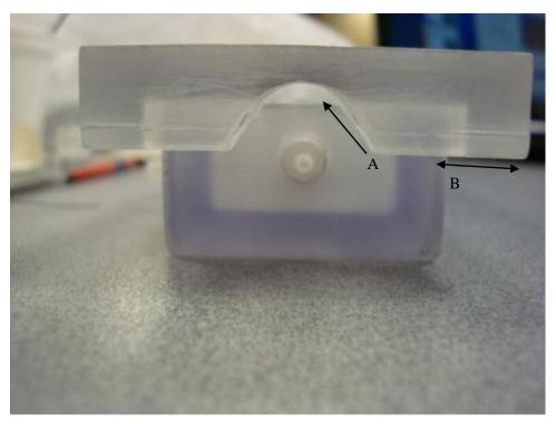
Figure 29: Arc cutout of the lid that enables gas exchange (A). The overhang of the lid can also be clearly seen here (B).
