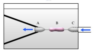
Figure 11: Open Cartridge Design 2 consists of plastic supports connected to a syringe needle (A) to hold the end of the tissue tube (B) while a syringe needle on the inlet (C) holds the other end.
