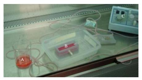
Figure 31: (A) Beaker containing media, (B) bioreactor chamber in plastic tray, and (C) pump being set up under a sterile fume hood.
