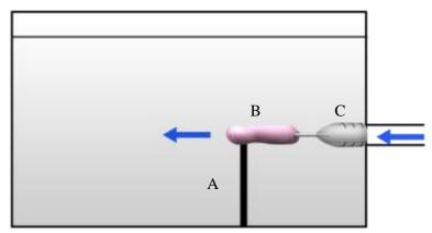
Figure 12: Open Cartridge Design 3 consists of a plastic arm with a round support (A) underneath the tissue tube (B). The syringe needle at the inlet (C) holds the tissue open.
