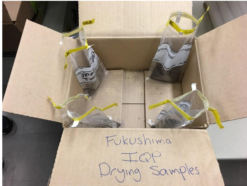
Figure 16: Samples drying by keeping them open to ambient air in one week (62.2 °F, 22% humidity and 1 atm)
