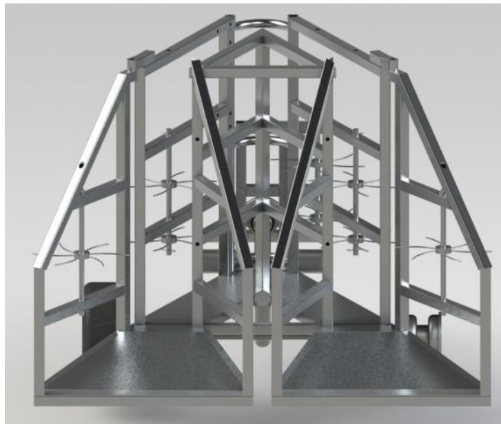
Figure 13: Feeder on Initial Binder
