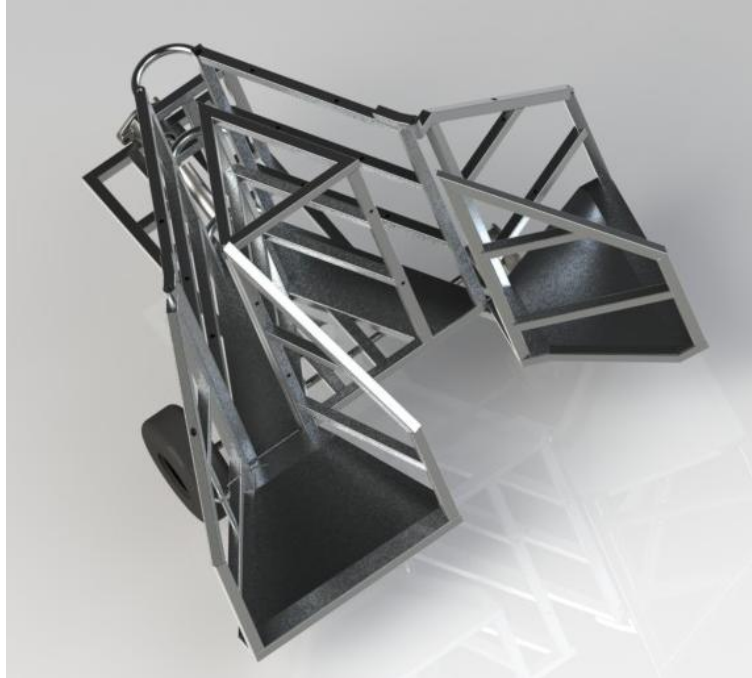
Figure 12: Replaceable Wings of Initial Binder
