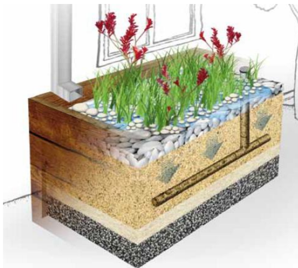
Figure 5; Raingarden diagram (Adapted from Melbourne Water)
