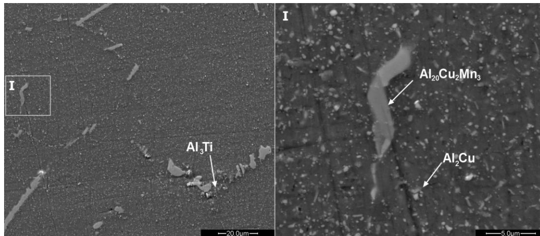
Figure 12. The inner microstructure of test samples at HTS
