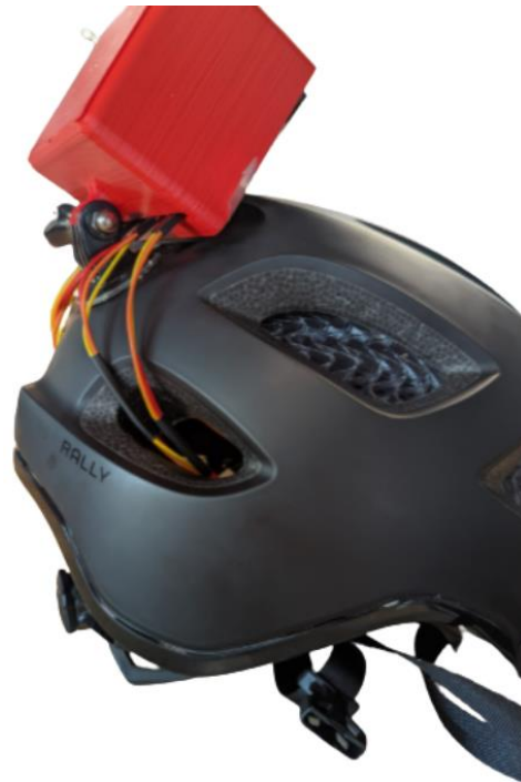
Figure 7: First Housing Unit Design
