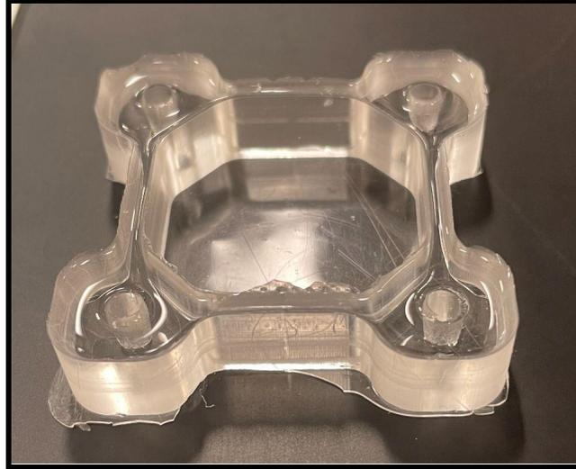
**Figure 3.** *PDMS dish before sterilization.*
