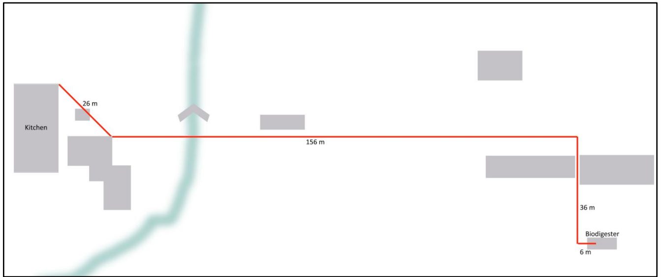
Figure 4.4-1: Piping Route to Kitchen
