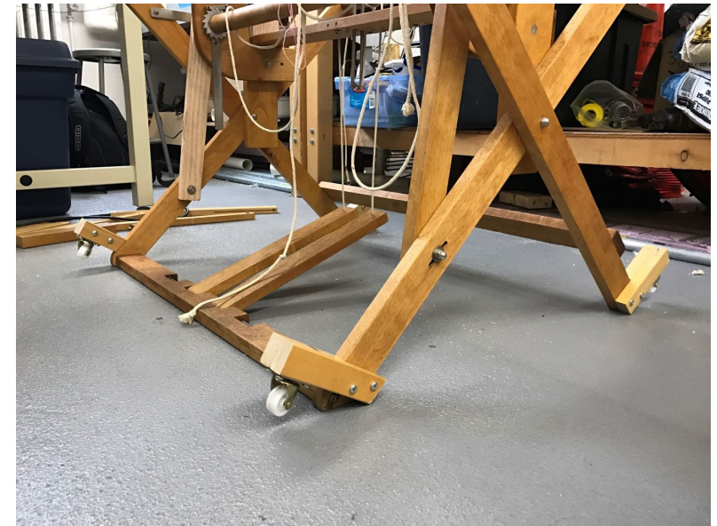
Figure 13. Loom with wheels in open position. Note that the wheels did not touch the floor when the loom was open.
